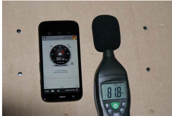
Figure 2 A smart phone with a noise app and a sound level meter, prior to calibration
