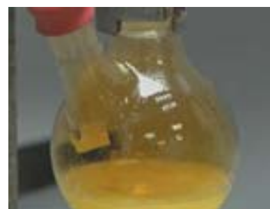
Figure 3.1 The reaction of benzene with nitric acid: brown fumes of \text{NO}_2 are formed as a by-product.
