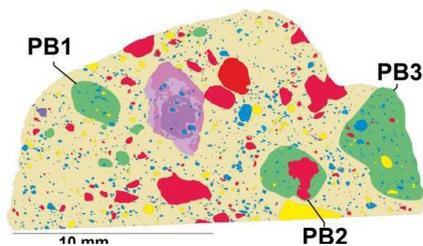
*Fig. 1: A false-coloured X-ray elemental map of a slice of NWA 7034 highlighting the diversity of breccia in breccia clasts (PB1, PB2, PB3).*
