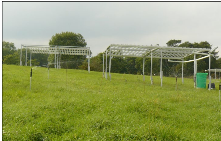
Figure 1: The rain shelters and irrigation system in operation at the RainDrop experimental site at Wytham, near Oxford.
